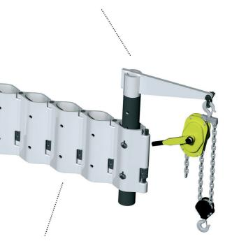
The JibFlex can be extended to reach out 7 m from the anchoring point. In this working radius, it can carry up to 150 kg. In a 3 m working radius, it can carry up to 500 kg. Please note that the working load limit (WLL) is defined as the payload plus the weight of the hoist mechanism.
